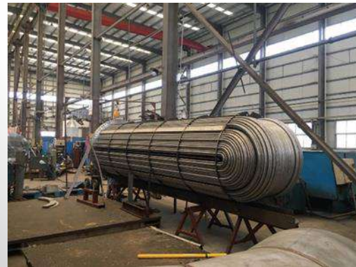
Stainless steel acid cooler tube bundles for Glencore Minara
