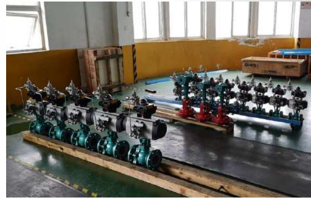
Control and Teflon lined valves for Glencore PASAR
