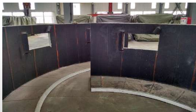
Rubber lined feedwells and piping for Paterson-Cooke Kumptor project
