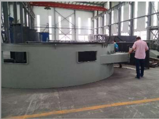
Rubber lined feedwells and piping for Paterson-Cooke Kumptor project
