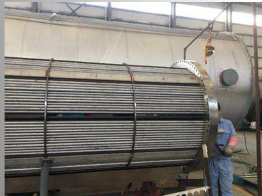
Stainless steel acid cooler tube bundles for Glencore Minara
