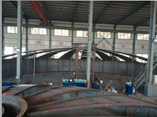
75' and 50' steel covers made in China for Ovivo projects in the US
