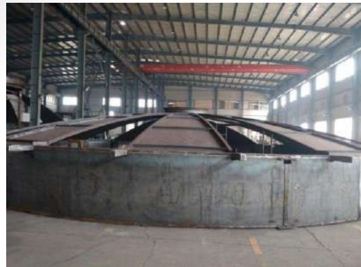
75' and 50' steel covers made in China for Ovivo projects in the US
