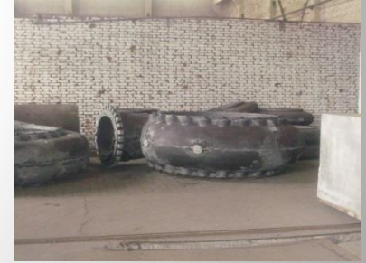
Pumps: cast, lathed and machined
