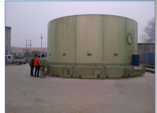
FRP reaction wells WesTech/GE
