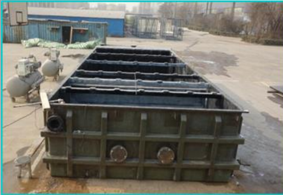
Settler tanks Areva/Technip
