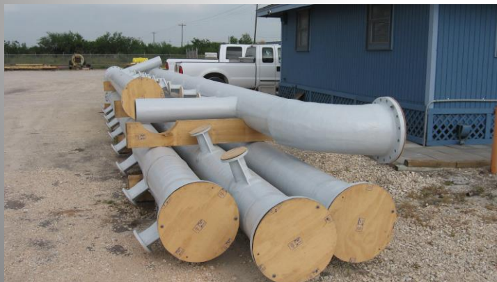
Fiberglass piping for SXEW plant
