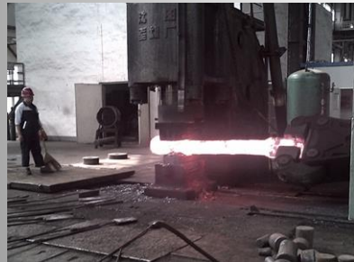
Pinions: Forged, heat treated and machined
