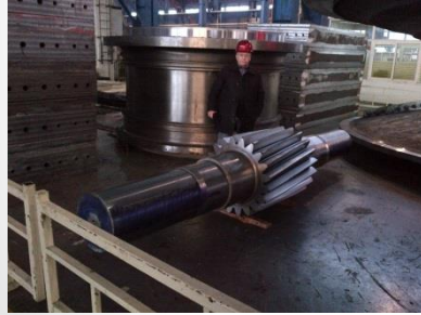
Pinions: Forged, heat treated and machined
